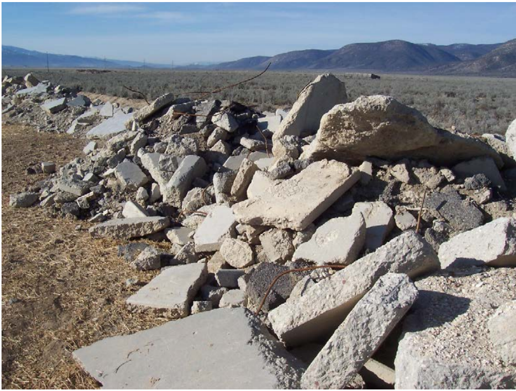
Waste asphalt intermixed with concrete debris
